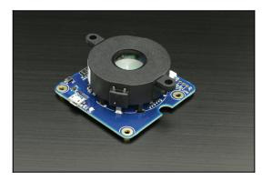
This device is a powerful USB buzzer. You can control both the frequency and the volume. There is even a way to preset simple beeping patterns.
