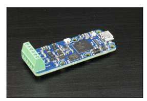
This device is an USB interface to query circuits through an I2C bus. If needed, the Yocto-I2C can act as a voltage source to power the external circuit with 1.8V, 3.3V or 5V. The I2C communication can be configured to 1.8V or 3.3V.
