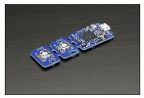
This USB device is an RGB LED driver. You can change color and luminosity of both LEDs. You can use it for simple signaling as well as for spectacular light effects.
