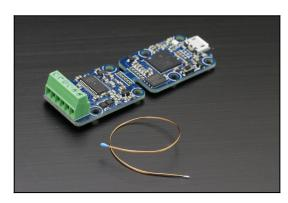
The Yocto-Bridge is a precision ratiometric analog/digital converter to measure over USB the very weak voltage produced by a load cell, as used in weighing scales, or any other type of strain sensor, or other sensor with a Wheatstone bridge output.
