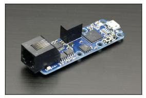
This device is a USB to RS232 adapter, that does not require a driver and does not install a virtual COM port.
