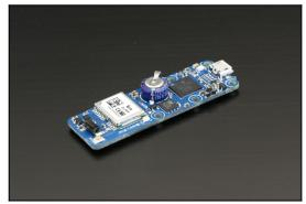
The Yocto-GPS device is a 32 channels receiver for GNSS signals emitted by GPS and GLONASS satellites, that enables it to determine the position of the receiver, its speed as well as the current time. The latitude and the longitude at any time can be recorded on the internal flash memory, in order to build a data history that can be retrieved later on over USB.
