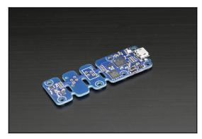
The Yocto-Altimeter-V2 device is a USB altimeter: it will give you an altitude estimate based on atmospheric pressure. The Yocto-Altimeter-V2 is precise enough to detect 10cm altitude changes. It will also give you the current pressure and temperature. Data can be recorded on the internal flash memory, in order to build a data history that can be retrieved later on over USB.
