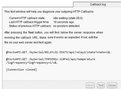
The result of the test callback with a Yocto-PowerRelay and a Yocto-Temperature
