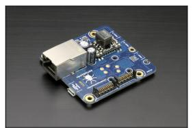
The YoctoHub-Ethernet is a Fast-Ethernet module which can host three Yoctopuce modules to access them remotely. It can be powered either by a Micro-B USB cable, or directly from the Ethernet cable (PoE compatible with the 802.3af standard).
