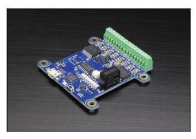
The Yocto-Maxi-IO-V2 device provides 8 digital I/O, electrically insulated from the USB bus. Each I/O bit can be configured individually as a simple input, an open-drain input (internal pull-up), a TTL/CMOS-like output, or an open-drain output (open collector).
