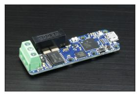
This device is a USB to RS485 adapter, that does not require a driver and does not install a virtual COM port.
